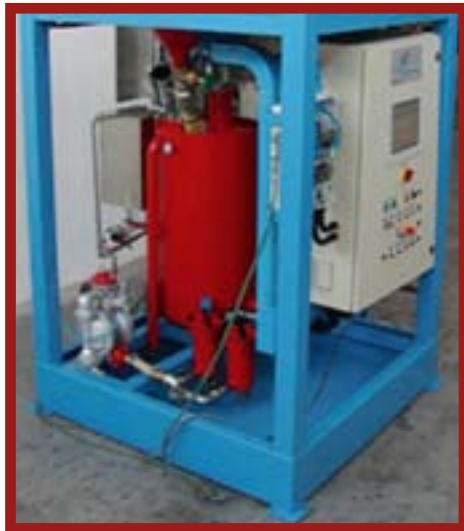
CPP Coating Preparation Plant
