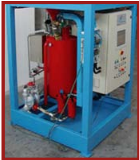
CPP Coating Preparation Plant
