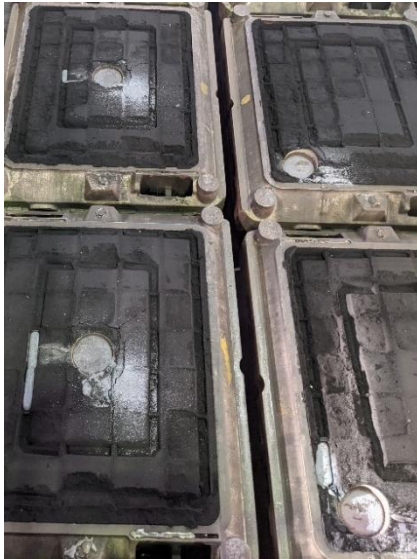
Figure 6: Inoculant buildup on top of the mould at the end of the pour
